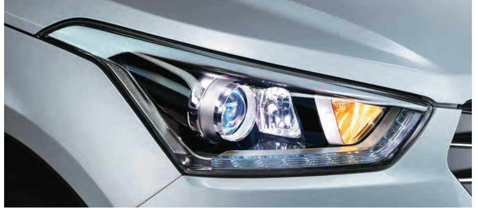
Bi-functional Projector Headlamps with LED Positioning Lamps
